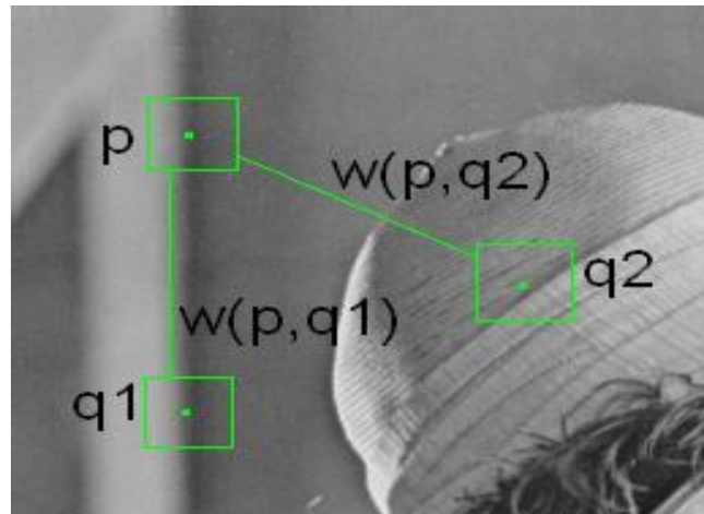
Figure 5: Example of self-similarity in an image. Pixels p and q1 have similar neighborhoods, but pixels p and q2 do not have similar neighborhoods. Because of this, pixel q1 will have a stronger influence on the denoised value of p than q2 .
